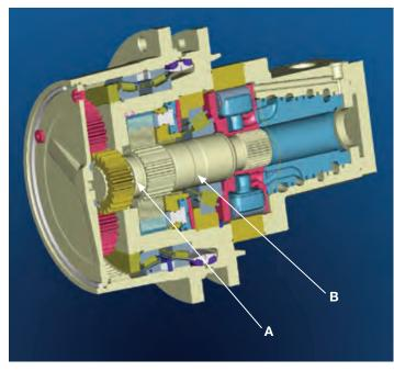
The combined gearbox (A) and motor (B) help maximize power output to the tracks. (C185 & C190 motor shown)
