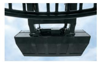
The see-through area on the cab roof provides a clear view to the bucket, even when it is positioned at full height.
