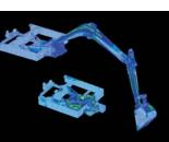
FEM(Finite Element Method) Durability of structure is proven through FEM(Finite Element Method) analysis and long term durability test.
