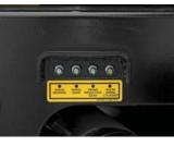
**Centralized Grease Fittings** service checks. Save time and money during routine maintenance.
