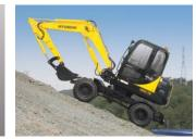
Gradeability 35 degree(70%) of high gradeability and long tumbler distance may be easier to work at slope area.
