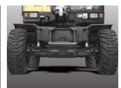
**Better Ground Clearance** Better ground clearance increases safety on rough ground.
