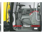
Sensitive Joystick and Easy Entrance New joystick grips for precise control have been equipped with 4 switches. Tilting tower combined with large door provides more space for gateway.
