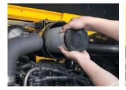
**Easy Change of Air Cleaner** The R55W-7A is fitted with durable plastic air cleaner for easy maintenance and quick service.
