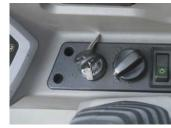
Anti Restart System The new system protects the starter from restarting during engine operation, even if the operator accidentally turns the start key again.
