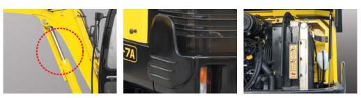
**Boom Cylinder Cover** to prevent cylinder damage.
