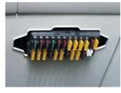
**Centralized Fuse Box** Fuse box is arranged on the rear of seat for easy service.
